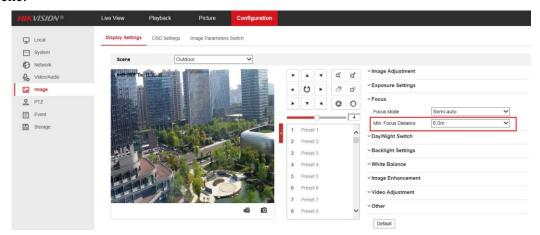
2) Setting an inappropriate Min. Focus Distance may cause slow or unfocused problems. To choose the right Min. Focus Distance according to the actual monitoring distance.
