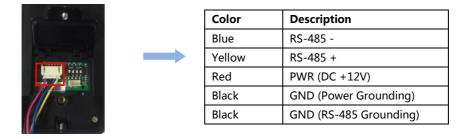
3. Correspondingly, there are RS485 interfaces in DS-K2600 series access controllers; you can find RS-485 interface at the same position in DS-K2601/02/04 access controllers, as pictures show:
