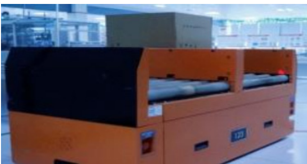
AGV Interworking with End-of-line Roller for Picking Materials
