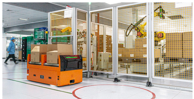
AGV Interworking with Case Seal Roller for Releasing Materials
