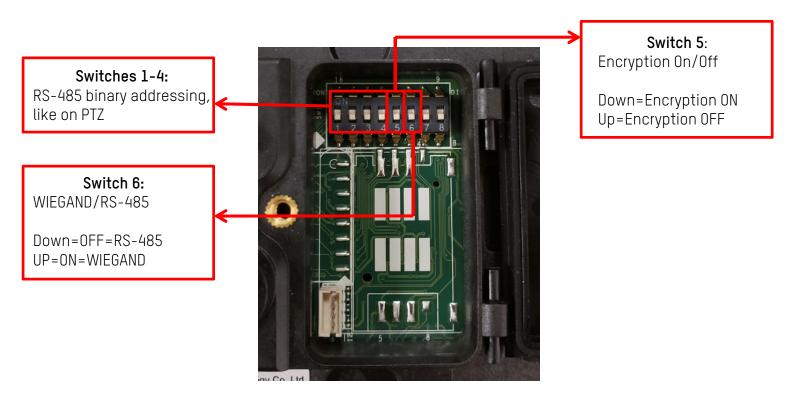
Figure 1, DIP Switch Location
