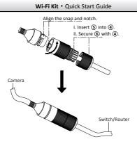
Figure 3-6 Waterproof Accessory Installation
