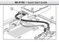
Figure 2-2 Connect Cables
