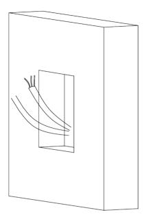
Figure 4-22 Drill the Installation Hole
