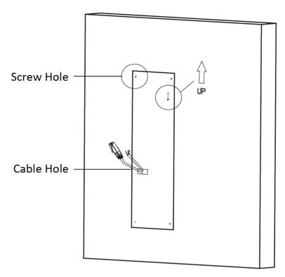
Figure 4-29 Drill Screw Holes
