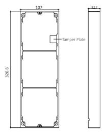
Figure 4-28 Mounting Frame
