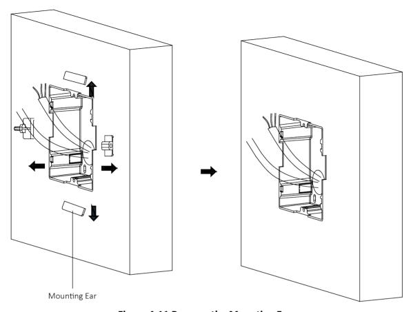
Figure 4-11 Remove the Mounting Ears
