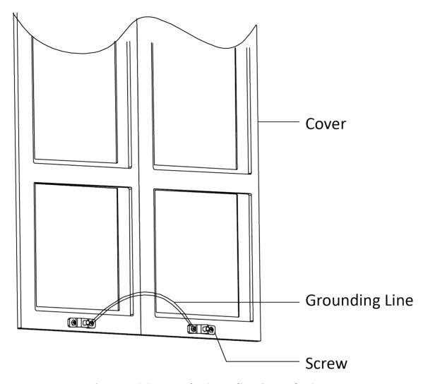
Figure 4-50 Connect the Grounding Line to the Cover
