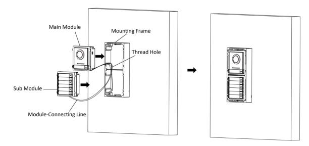
Figure 4-19 Insert the Modules
