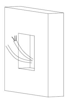
Figure 4-8 Drill Installation Hole
