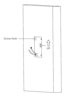
Figure 4-15 Drill Screw Holes
