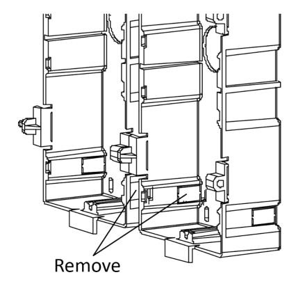
**Figure 4-55 Remove the Plastic Sheets**
