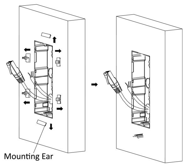
Figure 4-25 Remove the Mounting Ears
