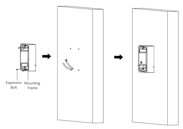
Figure 4-3 Fix the Mounting Frame
