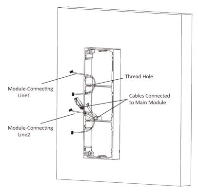
Figure 4-32 Placement of Lines
