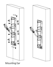
Figure 4-40 Remove the Mounting Ears
