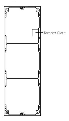
Figure 4-31 Mounting Frame
