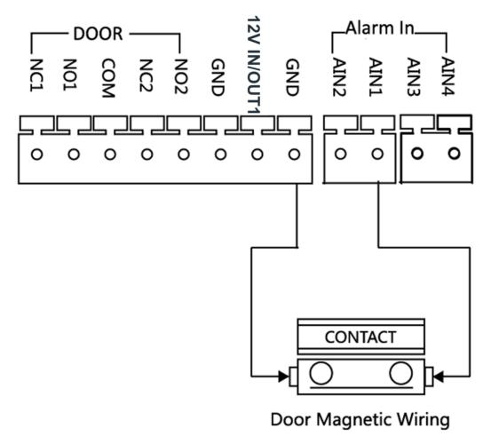
Figure 3-7 Door Contact Wiring
