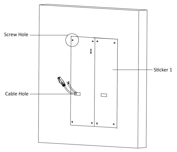
Figure 4-44 Drill Screw Holes
