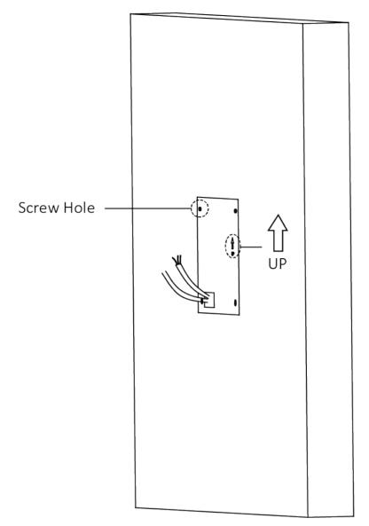
Figure 4-2 Drill Screw Holes
