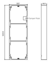
Figure 4-43 Mounting Frame
