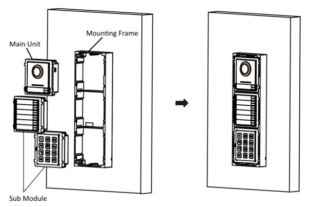
Figure 4-34 Insert the Modules into the Frame
