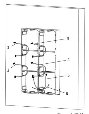
1,2,3,4 : module-connecting line (190 mm)
