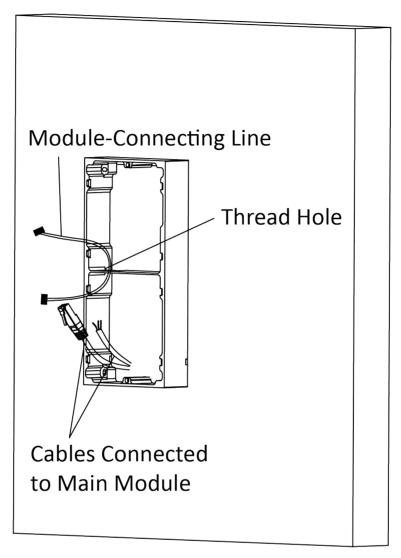
**Figure 4-17 Placement of Lines**
