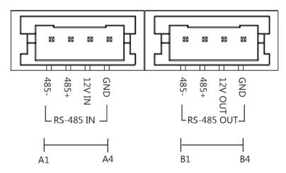
Figure 3-3 Sub Module Terminal (Except Touch-Display Module)
