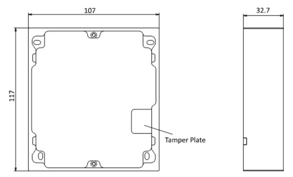
Figure 4-1 Mounting Frame
