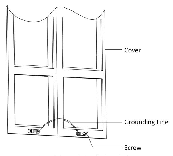
Figure 4-61 Connect the Grounding Line to the Cover
