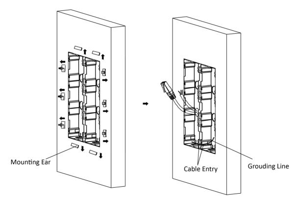
Figure 4-58 Remove the Mounting Ears
