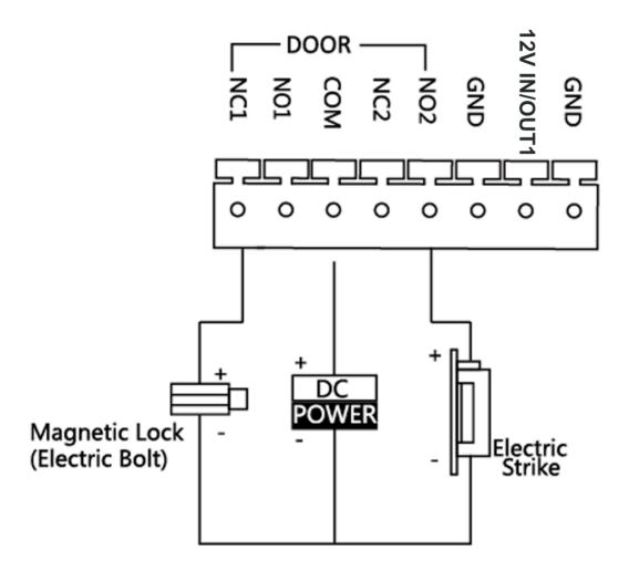
Figure 3-5 Door Lock Wiring
