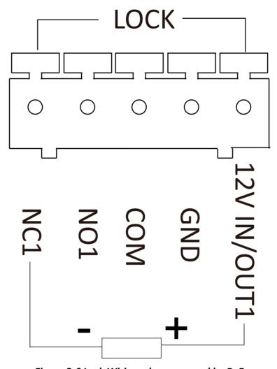
Figure 3-6 Lock Wiring when powered by PoE
