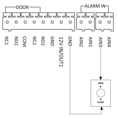
Figure 3-8 Exit Button Wiring
