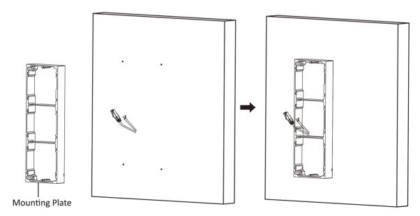
Figure 4-30 Fix the Mounting Frame
