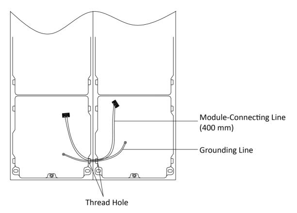
Figure 4-45 Place the Grounding Line and Module-Connecting Line
