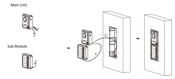
Figure 4-26 Connect Cables and Insert the Modules
