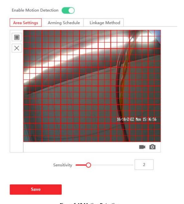
**Figure 6-13 Motion Detection**
