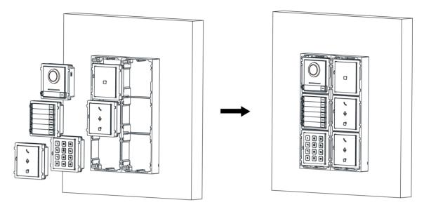
Figure 4-49 Insert the Modules
