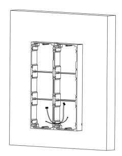
Figure 4-46 Fix the Mounting Frame
