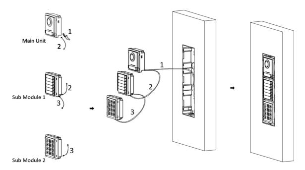
**Figure 4-41 Connect Cables and Insert Modules**
