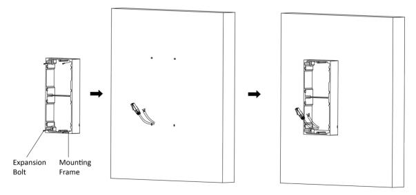
Figure 4-16 Fix the Mounting Frame
