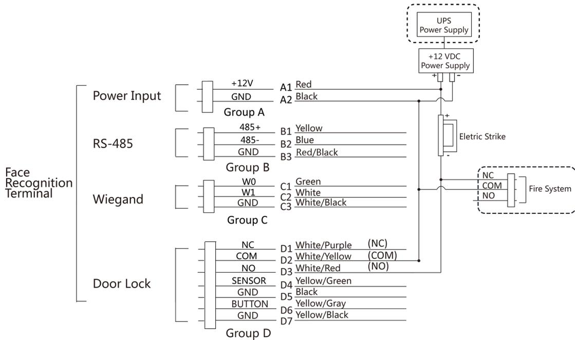
**Figure 4-7 Device Wiring**
