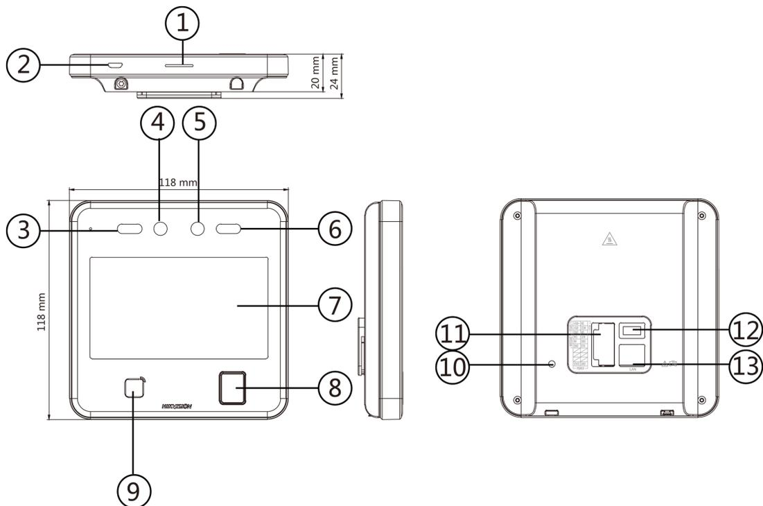
Figure 2-1 Face Recognition Terminal Diagram
