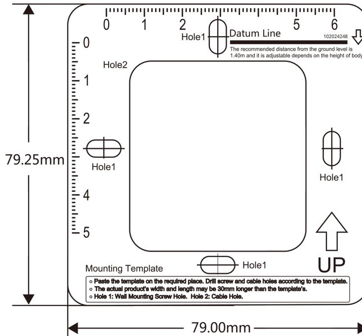
**Figure 3-1 Mounting Template**
