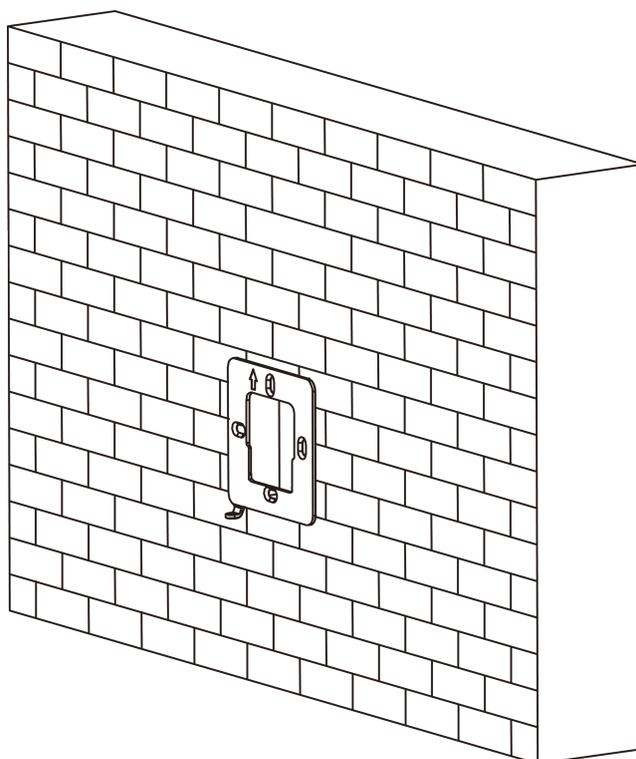
**Figure 3-2 Install Mounting Plate**
