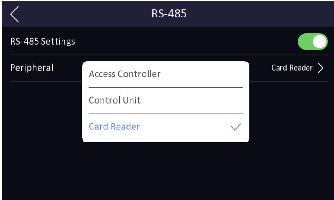
**Figure 7-6 Set RS-485 Parameters**
