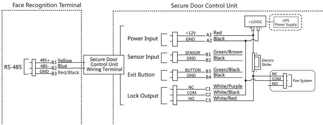
**Figure 4-8 Wiring Diagram**
