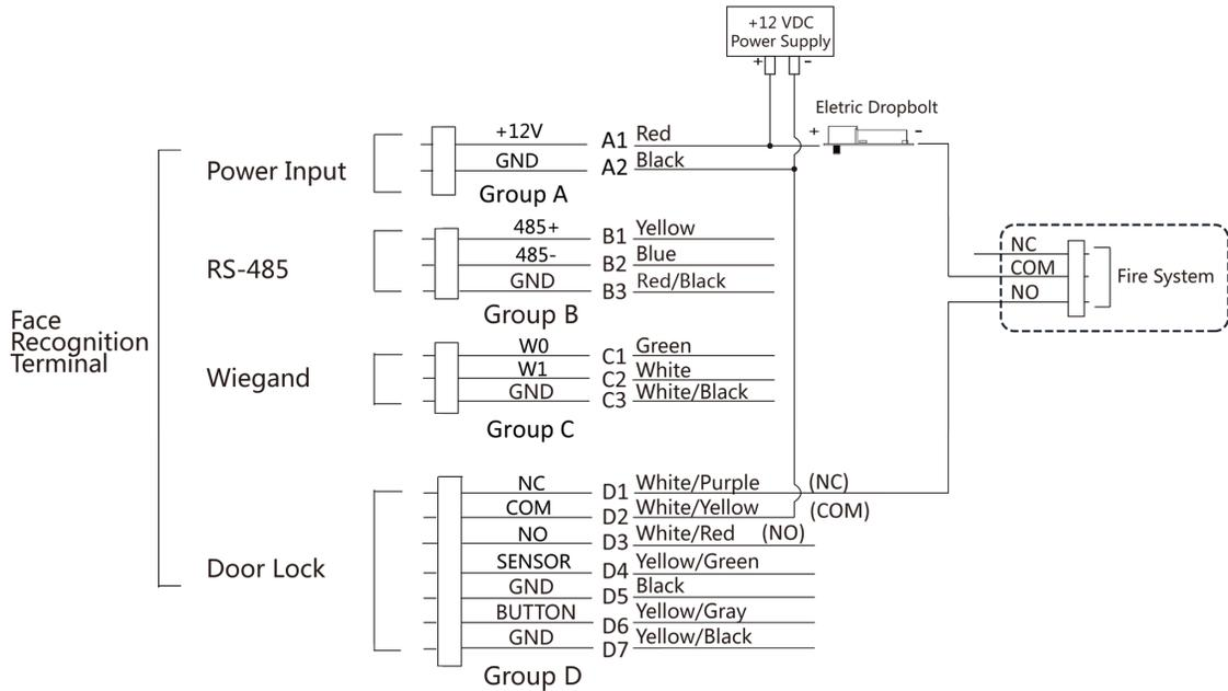
**Figure 4-5 Wiring Device**
