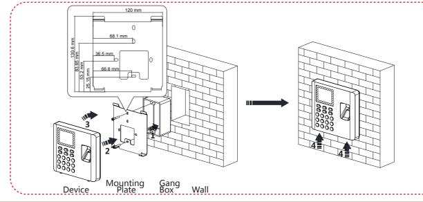
1. Install the gang box on the wall.
