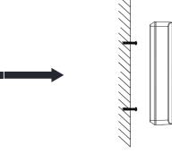
4. Align the 4 holes on the device plate with the fixed screws and hang the device on the wall.
