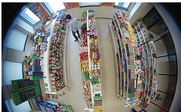
Fisheye cameras provide 360-degree views of retail environments using a convex lens.
