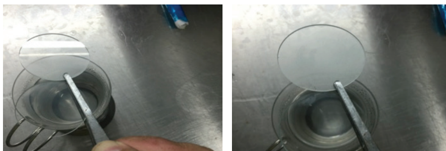
Figure 14 Test Result of Anti-Fogging Glass (Left) and Normal Glass (Right)
