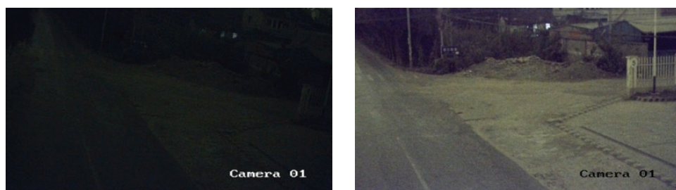
Figure 5 Night Vision Photo of f/1.5 Lens (Left) and f/0.95 Lens (Right)
