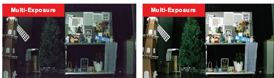
Figure 9 Multi-Exposure Off (Left) and On (Right)
