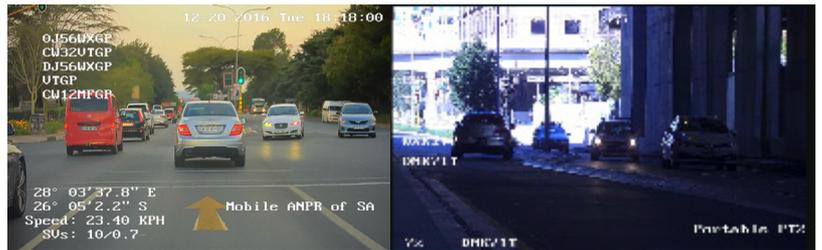
ANPR & GPS position & battery capacity overlay appear
