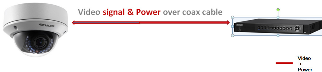
Figure 8, PoC 2.0 Wiring Topology
